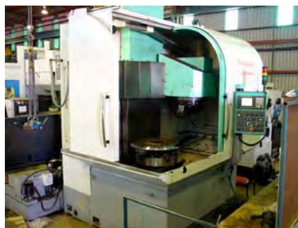
CNC Vertical Turret Lathe with 1250mm swing and live tooling for drilling & tapping.
