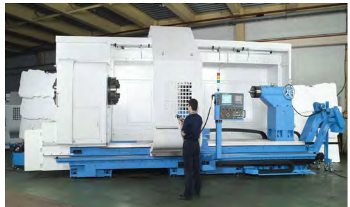
The L&L CNC shaft lathe with 900mm swing x 5200 between centres and a hydraulic steady is shown above left. The picture above right shows our Extreme swing Kinwa CNC lathe with 2500 swing x 4000mm between centres with 370dia hollow spindle, rear chucking and a 20kw milling head attachment.
