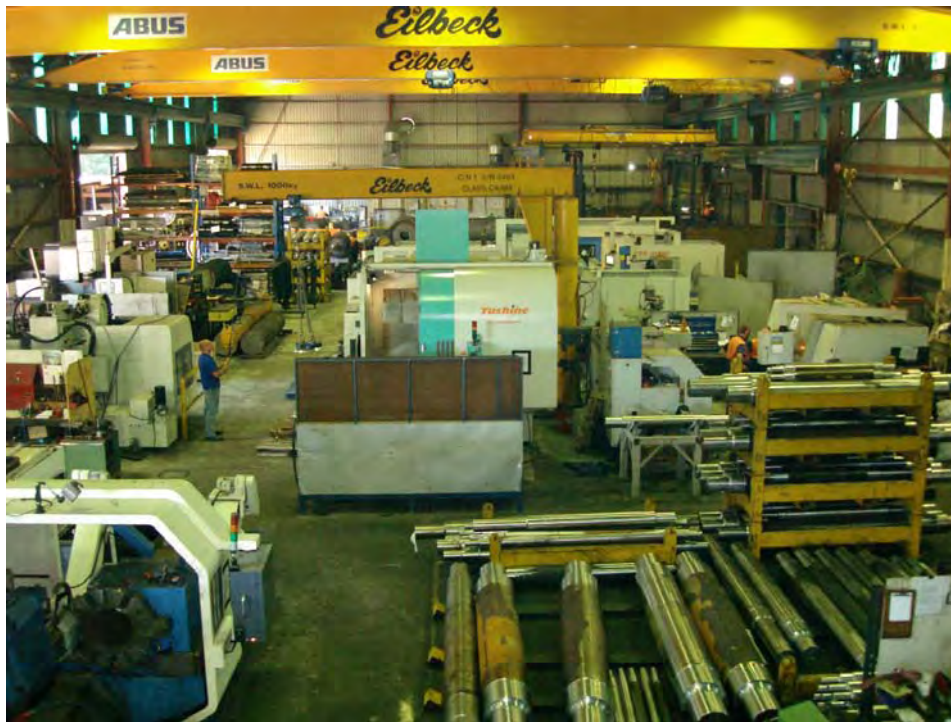
A part view of our West Gosford workshop which has a number of overhead cranes with up to 20 Tonne lift capacity.
