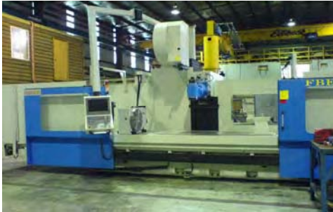
2 Eumach CNC Bed Mills – both with fully programmable heads for genuine five sided machining. The FBE4000 has 4000 long travel x 1000 cross travel & 1500 vertical travel and the FBE3000 is identical but with 3000 long travel. Both have a 500 diameter rotary table.
