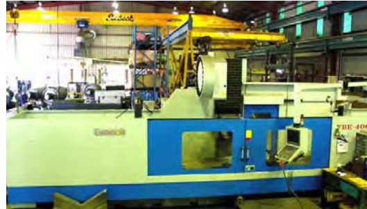
2 Eumach CNC Bed Mills – both with fully programmable heads for genuine five sided machining. The FBE4000 has 4000 long travel x 1000 cross travel & 1500 vertical travel and the FBE3000 is identical but with 3000 long travel. Both have a 500 diameter rotary table.
