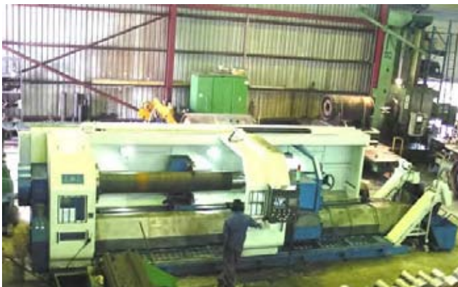
The L&L CNC shaft lathe with 900mm swing x 5200 between centres and a hydraulic steady is shown above left. The picture above right shows our Extreme swing Kinwa CNC lathe with 2500 swing x 4000mm between centres with 370dia hollow spindle, rear chucking and a 20kw milling head attachment.
