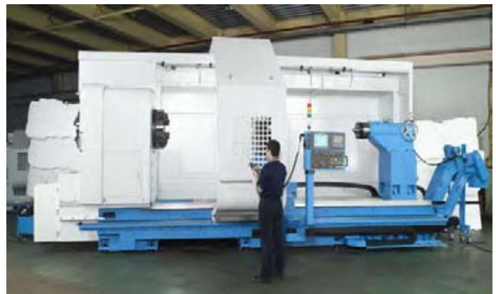
The L&L CNC shaft lathe with 900mm swing x 5200 between centres and a hydraulic steady is shown above left. The picture above right shows our Extreme swing Kinwa CNC lathe with 2500 swing x 4000mm between centres with 370dia hollow spindle, rear chucking and a 20kw milling head attachment.
